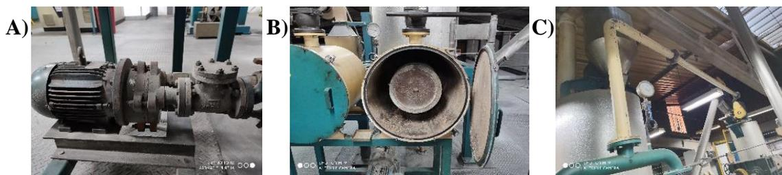
Fig. 1: PET extruder vacuum system. a) Air pump, b) Vacuum system, c) Pipe system.
