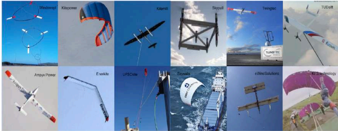
Fig. 3 AWE technologies in pumping kite mode under development. Source: Adapted from (Schmehl and Tulloch, 2019).
